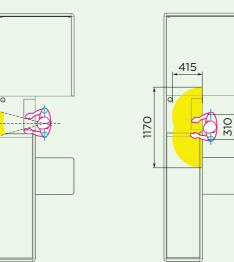
Arm movement area; field-of-view limits; field-of-view limits with trunk rotation.
